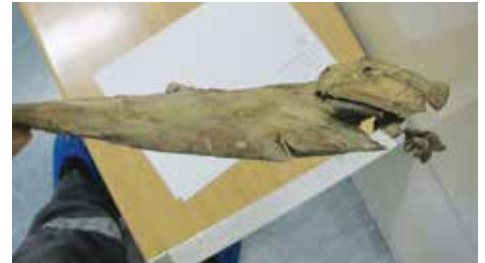
Several large items of sharp steel debris measuring up to 20cm x 30cm were recovered by the Tornar BOP Cleaner. This amount and size of debris could have resulted in permanent damage to the BOP if it had not been removed.
