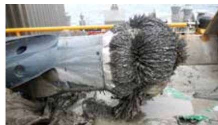
Figure 3. Swarf recovered by circulation magnet during first run.
