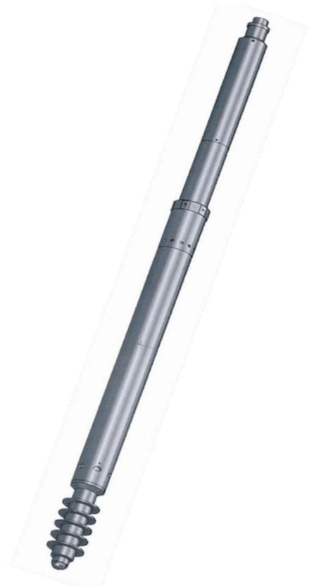
TASK/Launcher for side pocket mandrels (SPM's) utilizes a J-slot anchor with a disc assembly, which is set directly below the pocket in the SPM using a similar trigger finger to that used in kick-over tools. This gives a positive verification of depth and position. TASK/Launcher (SPM) is deployed with a stinger seal assembly in the bottom to close the equalizing ports in the assembly. When the pins are sheared, TASK/Launcher is activated and TASK is released to dissolve the scale.
