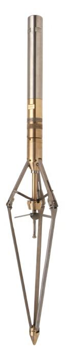
Production logging tools provide high resolution measurements of the fluid compositions and flow rates in the downhole environment that are used to evaluate well performance. A typical production logging toolstring is comprised of multiple sensors covering a range of physical measurements in order to identify fluid types, volumes and rates of their production or injection. Each of these measurements is digitised and recorded in order to create a comprehensive profile of the wellbore environment.
