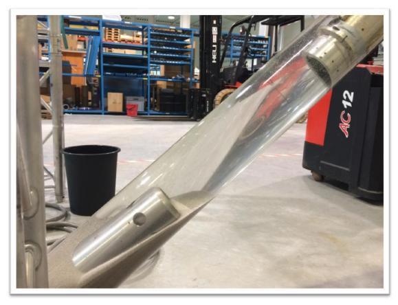
HEX plug in a deviated well with partial sand fill
