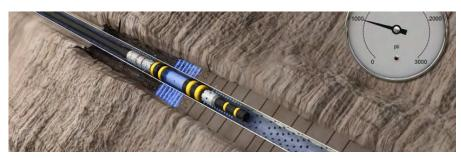
The first step of the operation was to run a Cement Bond Log to determine the optimum area to place the two barriers based on the Stronghold Barricade Systems operational window. The well was then perforated and the washing operations could commence.
