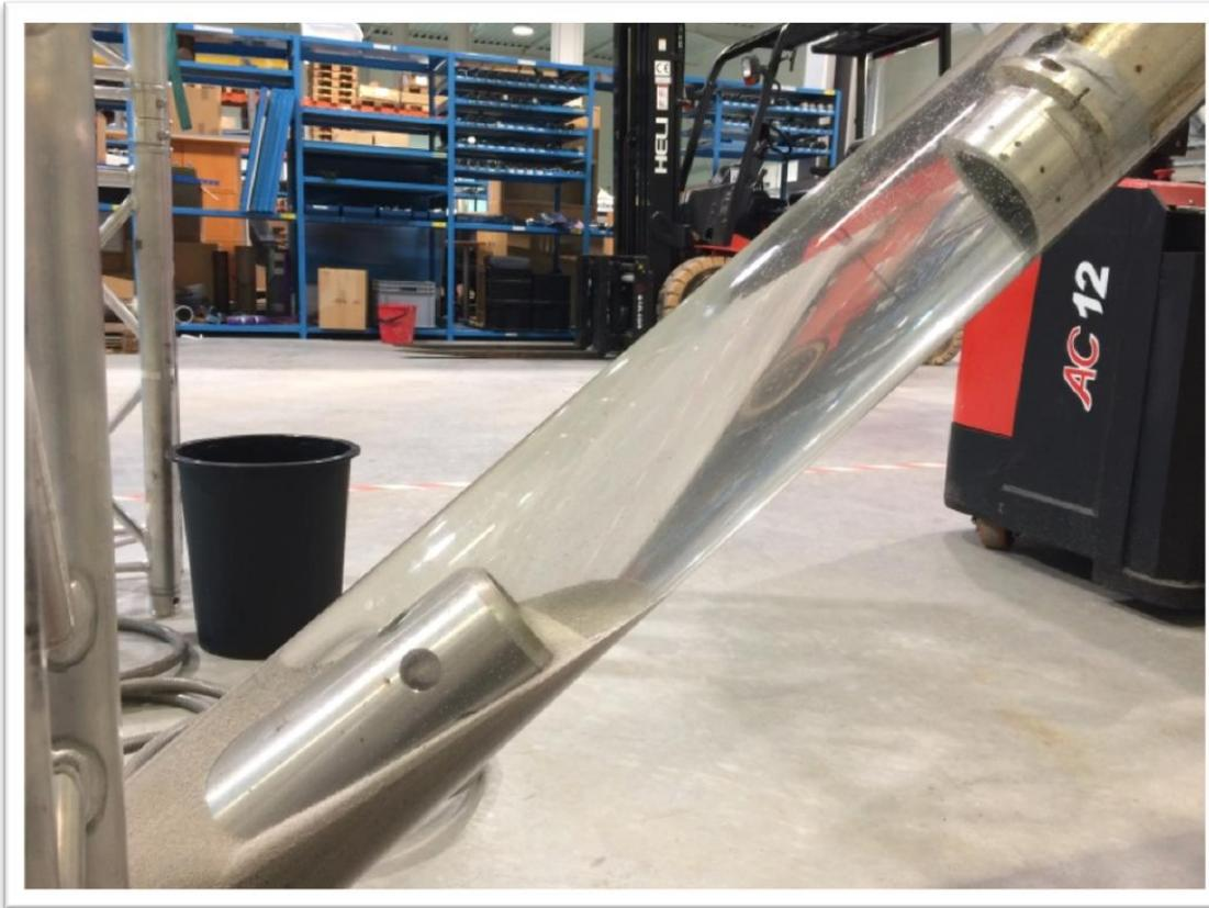
HEX plug in a deviated well with partial sand fill
