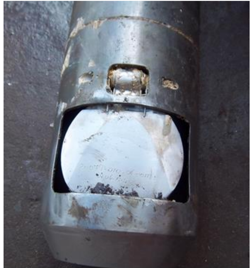
Flapper being held open by flotube
