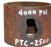
4" tubing 2 ½" PTC produced 1 hole appx. flow area 2.2 in 2
