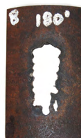
5" tubing 2 ⅝" PTC produced 2 holes 180° apart appx. flow area 3.75 in 2 (7.5 in 2 total)
