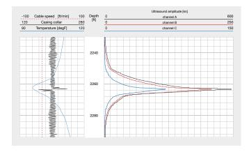
The diagnostic programme located a second unexpected leak at a tubing joint 2,300 ft above the gas lift system. This enabled the operator to complete the remediation program in a single campaign. saving time and resources
