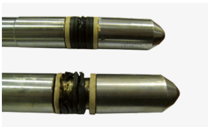
Retrieved GLV dummy (bottom) with its damaged seal. A healthy GLV replacement is shown (top).
