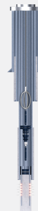
Data reception in memory, wireline or slickline conveyed
